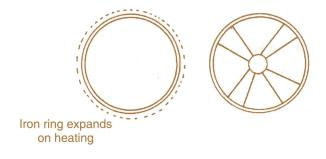
Fig. 14.10 Fitting iron tyre on wooden wheel
