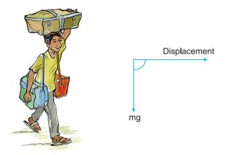
Fig. 13.3 No work done against gravity when a person moves on a level road carrying a heavy load on his head
