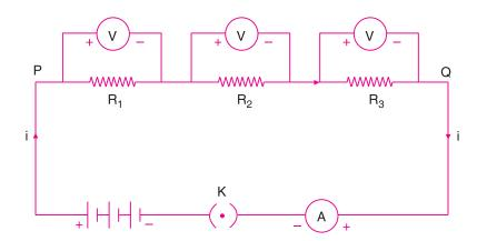
Fig. 16.7 Resistors in series
