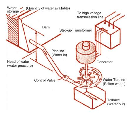
Fig. 12.7 Generation of Hydroelectricity
