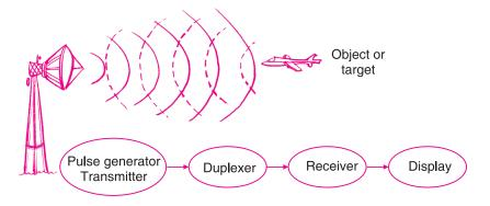
Fig. 18.8 A simple sketch of components of RADAR
