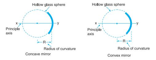
Fig. 15.11 Some important terms of spherical mirrors
