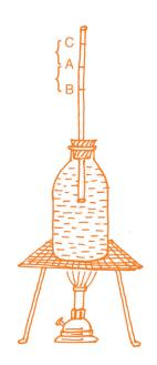
Fig. 14.7 Expansion of Liquid
