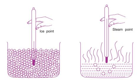
Fig. 14.2 Calibration of a thermometer
