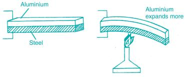
Fig. 14.6 The bimetallic strip bends on heating
