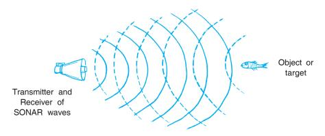
**Fig. 18.7** Working of SONAR: The continuous lines are used for transmitted SONAR waves and the dashed lines are used for reflected SONAR waves.
