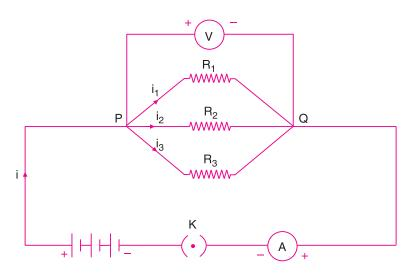
Fig. 16.8 Resistors in parallel
