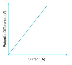
Fig. 16.6 (b) variation of voltage with current
