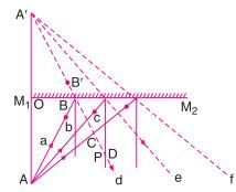
**Fig. 15.5** *Image formation by a plane mirror*
