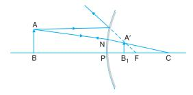
Fig. 15.15 Image formation by a convex mirror
