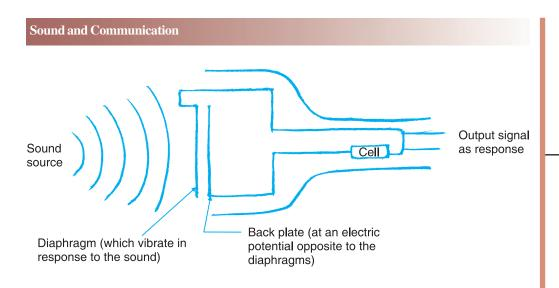
Fig. 18.10 (a) Structure of a condenser (capacitor) microphone
